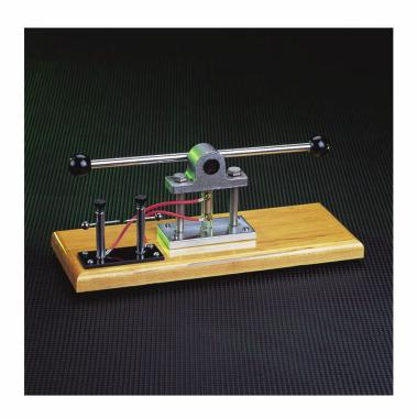
fingers across the terminals — you will feel a harmless tickle. Do this several times to assure yourself that you are generating a voltage, but on the last compression, do not touch the terminals. After a time lapse of 3 to 5 minutes, the charge will have dissipated. A final significant point is that piezoelectricity is a form of direct conversion of energy, from stress to electricity.
