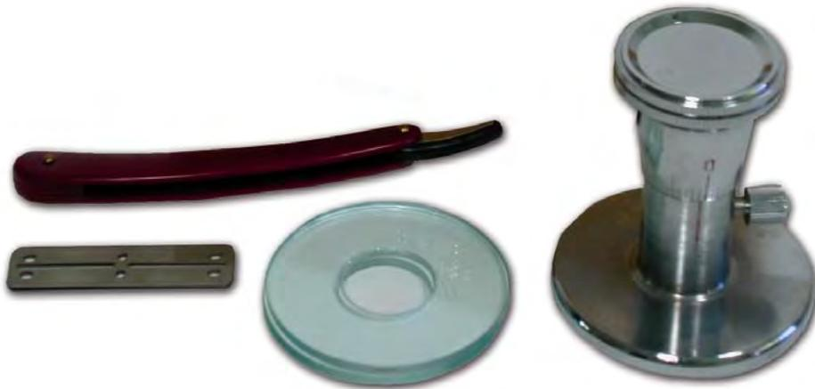
**Introduction:** A microtome is a device used to get an extremely thin slice of a sample. When cut thinly enough, most materials become translucent, making them perfect for viewing on a microscope. However, trying to cut consistently thin samples by hand is next to impossible, hence the need for a specific tool.
