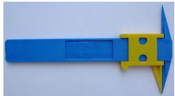
**Operation:** Your two point discriminator is very easy to use. It has a main section with a point on it, and a sliding section with another point. Printed on the main section is a scale, in millimeters.
