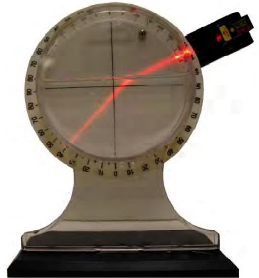
Water is a clear liquid, but has a certain property: it slows light down. A ray of light entering into a body of water is reduced to around 75% of the speed that same ray could achieve in a vacuum. This extremely abrupt shift in speed causes a ray of light to bend, which is known as refraction.
