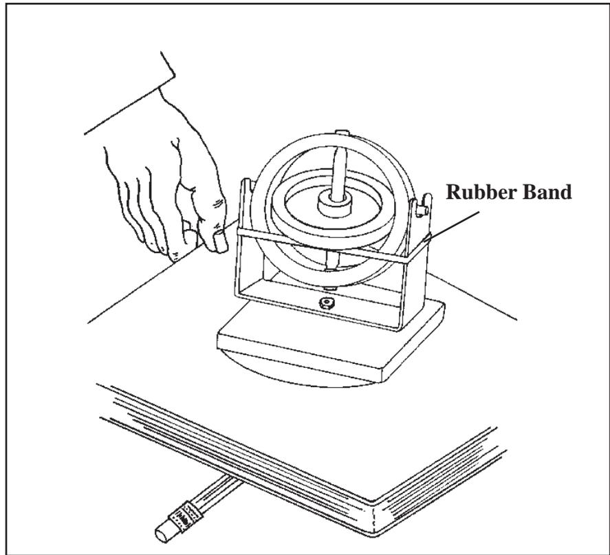
Figure 3 - Use elastic rubber band and pencil to simulate wave action on a boat.
