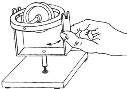
*Figure 2 -High Inertia. Rotor shaft horizontal.*
