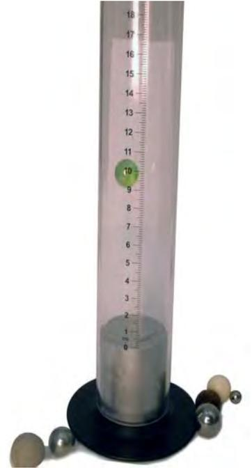
To use, choose a height on the scale and release one of the balls. Monitor it carefully and note the height of the rebound. Knowing the drop height and the rebound height, it is easy to calculate the coefficient of restitution.
