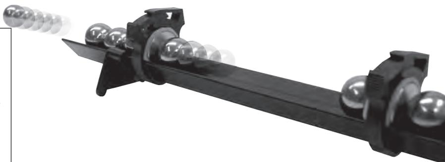
row. The impact of that ball kicks off the farthest ball on the other side just like Newton's Cradle. The released ball however has the energy of the magnetic acceleration propelling it faster than the original ball. This is possible because it begins its journey already a ball away from the original magnet. When this motion happens four times in a row, there is enough velocity built up to shoot a ball across a room!
