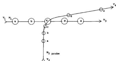
It was realized that each encounter with a planet was an elastic collision and could be used to both change the direction and increase the probe's speed. The "collision" does not involve contact with the planet's surface, but a passage through its gravitational field. The encounter is similar to the one dimensional example demonstrated above, even though it is really a two or even three dimensional collision.
