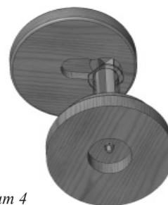
4. Slide plunger head over to the center of the cap block. The completed assembly is illustrated in *Diagram 5*.
