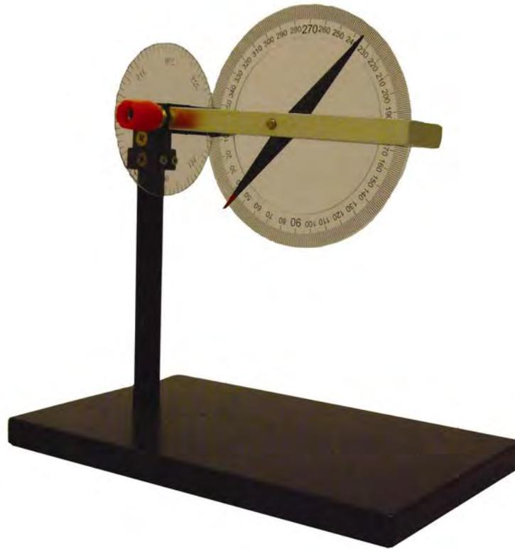
**Introduction:** Dip needles, also commonly known as dip circles, measure magnetic dip. When a magnetic needle is suspended vertically, it will form an angle with a horizontal plane. In effect, the needle represents the exact angle the earth's magnetic field makes at the latitude of the user.
