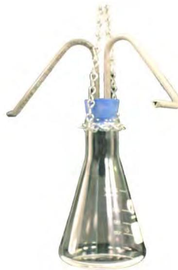
Make sure the unit is free to swivel. When you have secured the Engine, fill it about 1/3 of the way full. Check to be certain that the stopper is fitted firmly into the neck of the flask; if the stopper is too loose, steam pressure may cause it to fly off.
