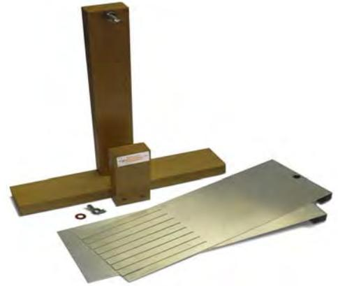
Note: this effect applies only for moving conductors. It is the motion that causes the induced current. Simply putting a magnet on a stationary conductor will not produce eddy currents.
