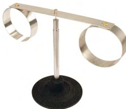
**Experiment :** Take your bar magnet and slide the North Pole through the closed aluminum loop.
