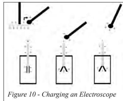
Figure 10 - Charging an Electroscope
