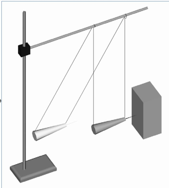
Place the block of wood on end so that it will stand 30 centimeters tall, and place it directly in front of the freely hanging dart. Mark the location of the block on the table using tape. Note that the dart will swing in the plane of the extension bar and the rod of the ring stand. The dart will also remain parallel to the table top throughout its swing. When releasing the dart, draw it back towards the ring stand the same amount each time, and release it without giving it a push.
