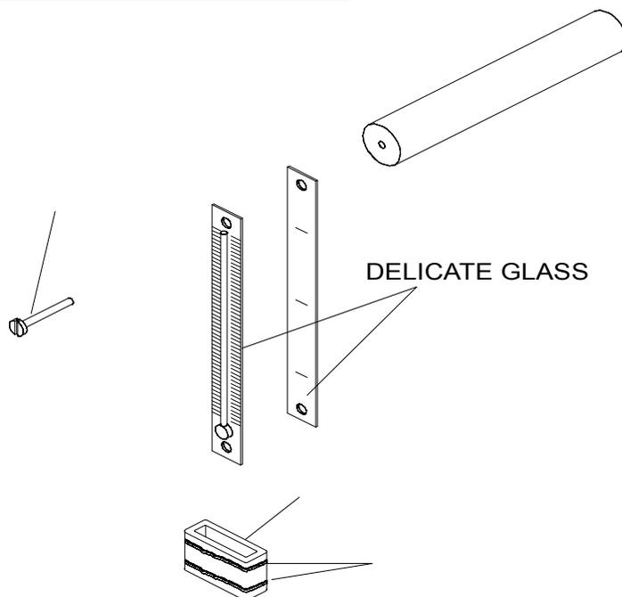
the same. The lowest reading will be on the wet bulb. Then with the aid of standard tables or graphs from the text, find the relative humidity using the temperature difference.
