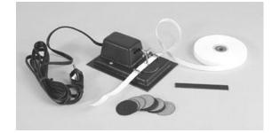
• To produce a position versus time record of moving objects using a mechanical striker and paper tape.
