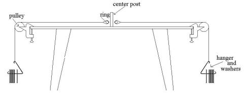
thread over the pulleys, as shown in the diagram below. Place the level on the table top and adjust the leveling feet on the legs until the table is level.
