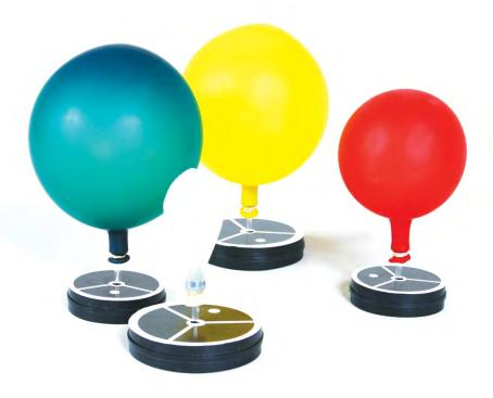
pucks on top of one another to quickly double the mass. The puck is now ready for use. When it is placed on a smooth flat surface, it will float on a thin cushion of air minimizing any resistance to movement due to friction. When choosing replacement balloons be mindful of the intended use. If the balloon is too large, collision experiments may not work because the balloon may collide with the obstacle
