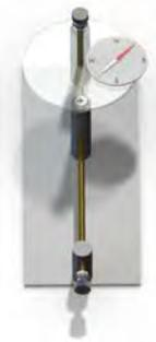
9. With current flowing, there will be little noticeable effect on the compass needle.
