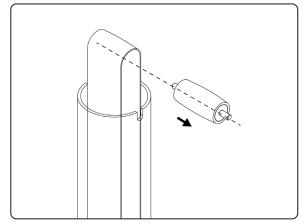
Remove the upper pulley from the belt and set aside. Allow the belt to fall into the column.
