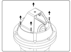
Remove the upper comb assembly by unscrewing the four indicated screws.
