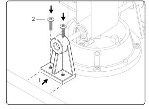
Replace the lower pulley arm and screw it back into the base.
