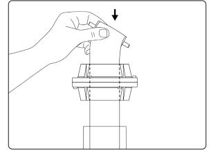
Angle the pulley and pass it through the black collar. Do not drop the pulley.
