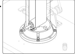
Settle the support column into the base.
