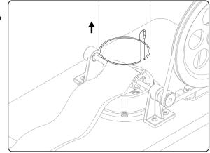
Lift the support column off the machine and set aside.
