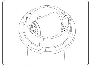
Settle the upper pulley into the notches on the black collar. Ensure the collar clicks into place on the support column.
