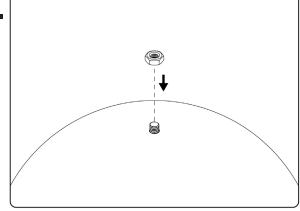
Screw the top nut back onto the dome.
