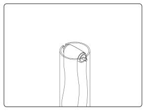
Settle the upper pulley dowels into the notches on the support column.
