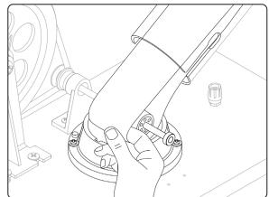
Reach into the bottom of the column and grab the belt. Stretch it over the lower pulley. Remove any folds or twists.
