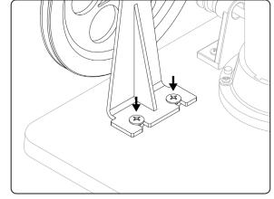
Tighten the screws on the base of the generator, securing the large pulley in place.
