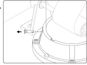
Use a flathead screwdriver to remove the two black pins found on the lower collar at the base of the column.
