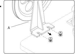
Loosen the two screws on the base of the generator and slide the large pulley (A) into place underneath them. 4.
