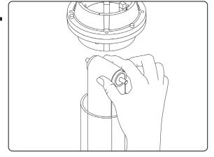
Remove the black collar, ensuring the pulley doesn't fall into the column.
