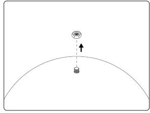
Remove the top screw from the dome and set aside.
