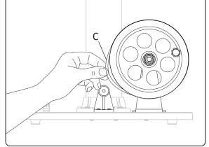
Carefully grasp the O-ring (C) found on the large pulley.
