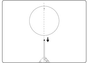
Place the dome on top of the upper comb assembly, ensuring the bolt pokes through the hole on the dome.
