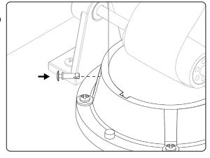
Insert the two black pins back into the lower collar.
