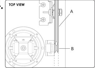
Align the large pulley (A) with the small pulley (B).
