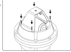
Screw the upper comb assembly back into place.
