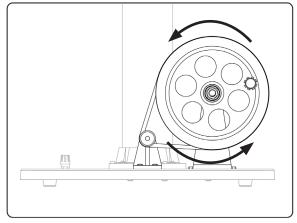
Turn the handle several times to ensure the pulleys are properly aligned. Adjust the placement of the large pulley as needed.
