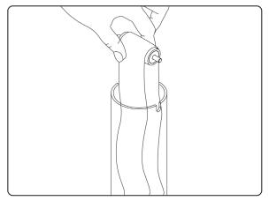
Hang the replacement belt on the upper pulley and lower both into the support column.
