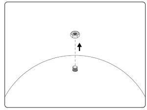
Before unboxing, remove the top screw from the dome and set aside.
