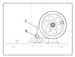
Stretch the O-ring (C) until it fits over the small pulley (B), as shown.
