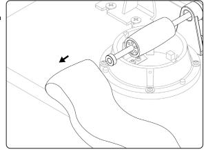
Remove the belt from the lower pulley and discard (replacement) or clean (maintenance).
