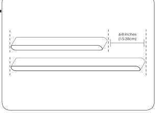
If replacing the belt, stretch the new belt an additional 6–8 inches several times.
