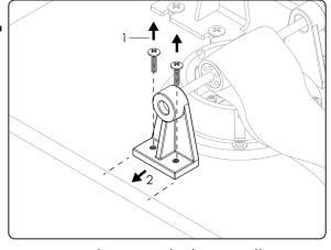
Unscrew and remove the lower pulley arm.
