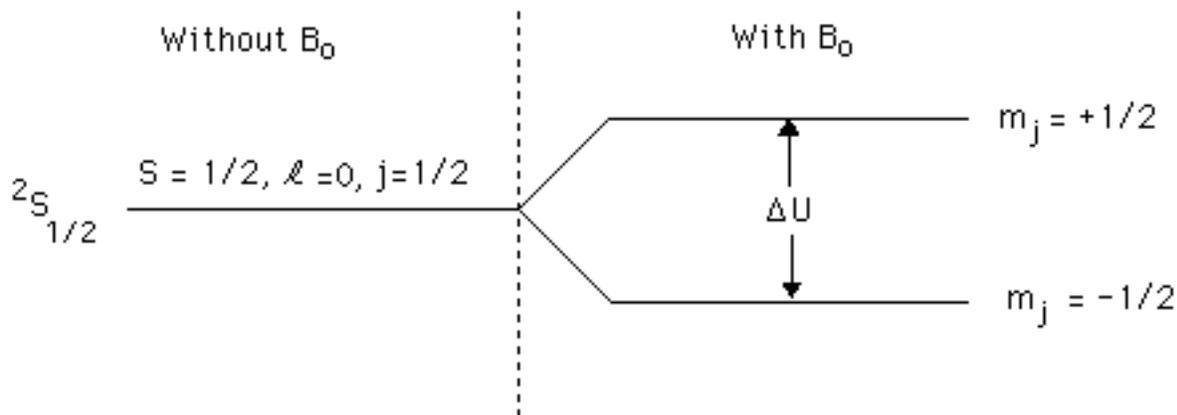
Figure 4. Energy level splitting in an atom or molecule with one optically active electron outside a closed subshell-pure spin angular momentum state:  $s = 1/2, l = 0, j = 1/2$  placed in an external magnetic field.
