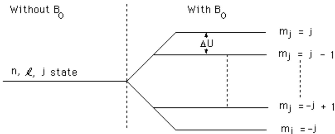
Figure 3. Energy level splitting of a multielectron atom or molecule with electron spin placed in an external magnetic field  $B_0$
