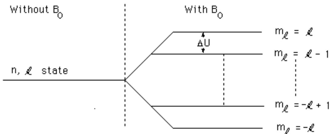
Figure 2. Energy Level splitting of a single electron (no spin) atom placed in an external magnetic field  $\mathbf{B}_0$
