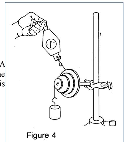
Wrap cord counterclockwise in the groove of the D wheel, or axle, and wrap the A cord clockwise in the groove of the A wheel. Tie a loop at the free end of each cord. Slip the spring balance on the cord loop from the A wheel. Hook a 500g weight on the loop from the D wheel (axle). Allow weight to rest on lab bench. Holding the balance vertically, above the wheel and axle, pull upward and lift the weight off the lab bench. Note the scale reading ; it should be 168. This figure was
