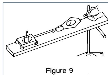
Adjust elevation of the inclined plane to 17.4cm, and pull the carriage up the incline using the spring scale. See Figure 9. Record scale reading. Repeat with 100, 200, 500, and 1000g weights.
