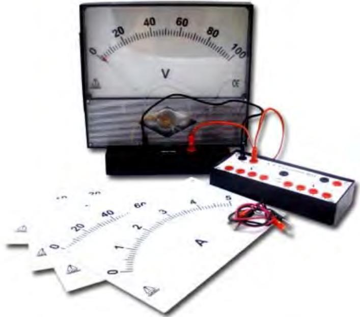
**Operation:** your demonstration meter requires a low voltage power supply to operate. There are a number of ways you can use the equipment. Using the included cords, you can attach your power supply directly to the meter through the jacks on the base. However, for a greater range of currents and potentials, you can use the extension box. Using a voltage power supply, you can generate 3V, 10V, 30V, or 100V. Alternatively, you can produce 10A, 5A, 1A, or 0.1A.
