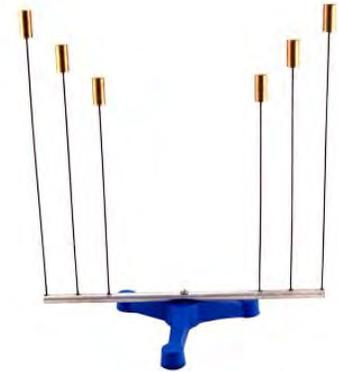
**Description:** Our set provides a simple and fun demonstration of resonance. The device consists of an aluminum tube bolted to a steel base. Attached to the tube are six spring steel rods in three lengths, with an equal brass weight on the end of each. They are arranged with the shorter rods near the center and the longer rods on the outside.
