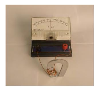
It is also possible to create a current by leaving the conductor stationary and subjecting it to a moving magnetic field. Using the same coil as the above experiment, place a bar magnet in the center. Hold the coils as still as possible and move the magnet up and down. Record the voltage. See figure below:
