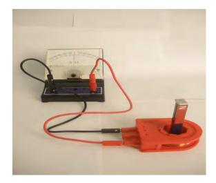
Changing the polarity of the magnet or the direction of the coil will change the way the galvanometer deflects. Magnets have a north and South Pole, and the coils are wound clockwise or counterclockwise. To change either value, simply turn the magnet or coil upside down.
