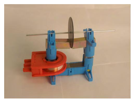
Spin the disc using the axle so it rotates quickly. While it is spinning briefly connect the coil to a DC power supply delivering 6 volts. Note pre set up this so that when you have the disc spinning all you need do is switch on the 6-volt supply.
