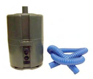
**Description:** Air tracks are a useful piece of laboratory equipment, but they are of little use if there is no source of air present. For this reason, it is essential to attach an air supply to the air track. The air supply operates like a vacuum pump in reverse; it discharges pressurized air. This air then enters the air track, escaping from the small holes throughout its length. This creates a cushion of air along the skin of the air track that is powerful enough to lift gliders.
