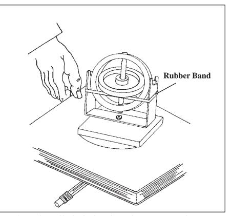
Figure 3 - Use elastic rubber band and pencil to simulate wave action on a boat.
