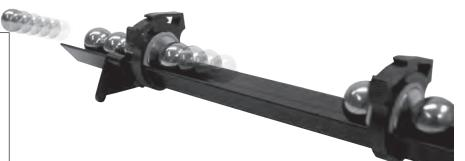
ramp allows for a reproducible initial velocity for performing experiments. As the first ball nears the first magnet, the magnetic force begins to pull the ball towards it and increases its velocity. The force that the magnet has on the ball increases exponentially as the ball gets closer and closer to it. This is because the strength of the magnet at a given point is equal to the inverse of the square of the distance to it.
