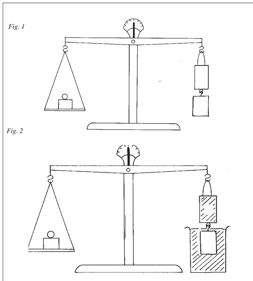
Another way to use this apparatus is illustrated below. Fit the solid cylinder inside the bucket as shown. Submerge both cylinder and bucket in your container of water. Use the length of dacron line to attach the handle of bucket to one arm of the triple beam balance and weigh both pieces by counterbalancing with the appropriate number of weights.
