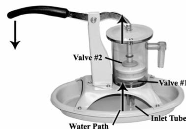
Step 2: Pull the pump handle back up. This causes the water pressure to close valve #1 and open valve #2. The water is pushed through valve #2 and above the plunger.
