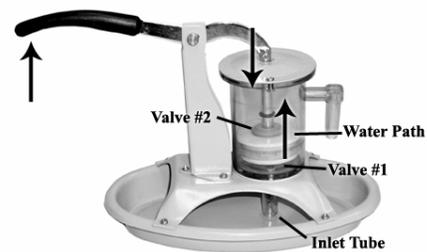
Step 3: Push the pump handle down again. As in step 1, Valve #1 opens and Valve #2 closes. This forces the water trapped above the plunger to be pushed out of the outlet tube.
