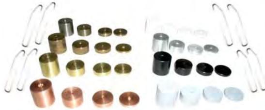
**Description:** Use this set to determine the specific gravity of a material by graphical methods. Fifteen individual determinations of specific gravity per material can be made. These results are plotted on a graph, the slope of which is the specific gravity of the material.
