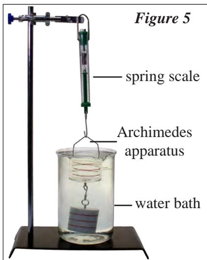
tainer of water. Since the cylinder no longer fills the bucket and the bucket is now submerged, it naturally fills completely with water. See **Figure 5**.
