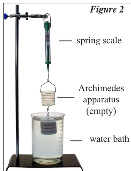
top surface of the cylinder is just below the surface of the water. Measure the weight of the apparatus. It will appear as though the cylinder and bucket weigh less in water. See **Figure 2**.
