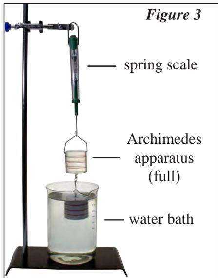
original value. This demonstrates that the weight of the water in the bucket is equal to the weight of the water displaced by the cylinder.
