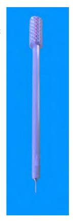
Due to the length of the probe, it may take some time to equalize to the temperature of your sample. Generally, if you require a more precise measurement it will take more time to equalize.
