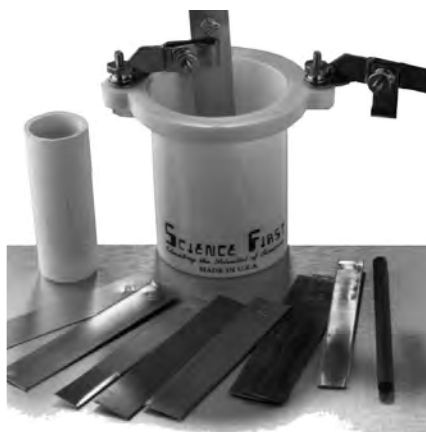
Photo shows one bracket swung outward. To use, position both brackets so electrodes protrude into jar.
