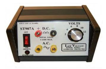
**Introduction**: power supplies are a staple of laboratory equipment. They are particularly useful for instruments that require power in amounts other than what a wall socket can supply; either low voltages or very high voltages. Our power supply is a **low voltage** design, useful for a variety of small apparatus or when batteries are not available.
