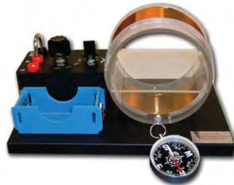
**Operation:** For your set you will need one D-cell battery, which is placed in the holder. There is a U shaped wire that must be secured in place to allow current to flow. You will notice two knobs: one of them switches between the three coils: one of 100 turns, 200 turns, and 400 turns. These three coils all occupy the acrylic cylinder. The second knob is used to tune the device. The coils of wire surround a horizontal acrylic plate. A compass is included in the set.
