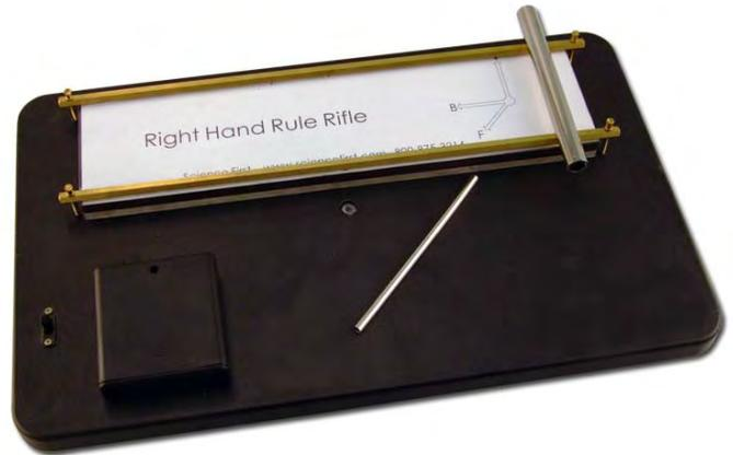
The right hand rule is named after the grip position used to determine the magnetic field. Grip the roller in your right hand with your thumb pointed in the direction current flows. Your fingers will wrap around the roller in the same direction as the magnetic field.
