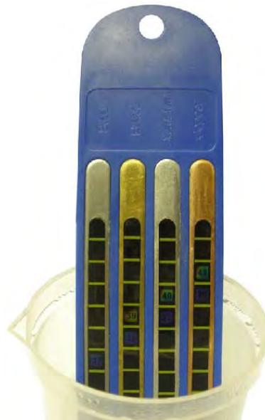
To use, simply **put on safety goggles**, take hot water that has been boiled, let it sit for 5 minutes and immerse the ends of the metal strips into the water. See warning below. Watch as the thermometers indicate the temperature of each metal. Which conducts heat the best?
