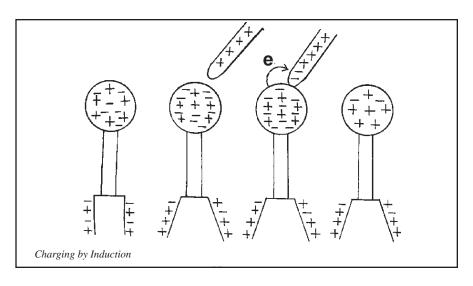
Removing the charge rod causes the electrons to return to their original positions. The leaves collapse.
