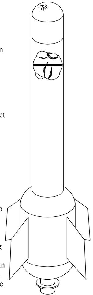
An inverted nose cone, securely taped, can carry a parachute -- or even a ball. The bottom 10cm of a 2 liter bottle, well taped to the top of the pressurized bottle, has lofted a real soccer ball!
