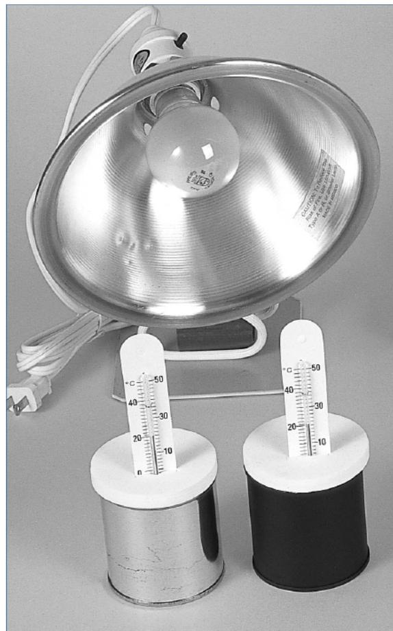
Then turn the light on. Record the temperature from each container every minute for 10 minutes then turn the light off again. Continue recording the temperature from each container every minute for 10 more minutes. Chart your data with temperature on the vertical axis and time on the horizontal axis.
