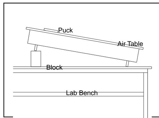
experiment when he dropped balls of various masses from the leaning tower of Pisa? Repeat the experiment moving the puck down hill in increments of 30 cm. Make a table of average speed and distance traveled. Can you determine the acceleration of the puck from your data? Try the experiment with a triple mass puck.
