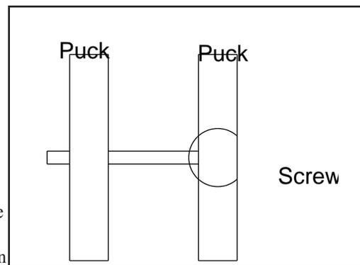
To carry out an experiment to determine whether a rolling or sliding disk would reach the bottom first, you will first need two small size pucks and a stop watch. Raise one end of the Air Table about 2 centimeters. Connect two pucks as shown in figure 11. Use a long screw to connect the pucks. With the air off, allow the pucks to roll down the incline. Next, with the air on, allow the pucks to slide down the incline. Time the motion of the pucks each time.
