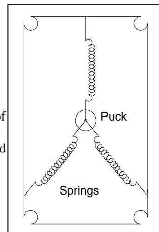
Move the springs to other positions on the table and draw vector diagrams of the forces acting on the puck. How would your results be affected if a more massive puck were used? What would be the effect of carrying out the experiment on a tilted table? Could you carry out this experiment using two springs with gravity as the third force component? Try it.
