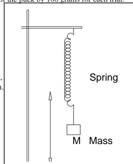
Suspend one spring and hang a 20 gram mass from its free end. Pull the mass down 10 cm. and release it. Time each oscillation to find out if the time for each complete oscillation (period) is the same or different. Can you explain your results? Pull the mass down 20 cm and release it. How does the period compare with that in the previous example? Try several different displacements until you can determine the relationship between the period of oscillation and the initial displacement.
