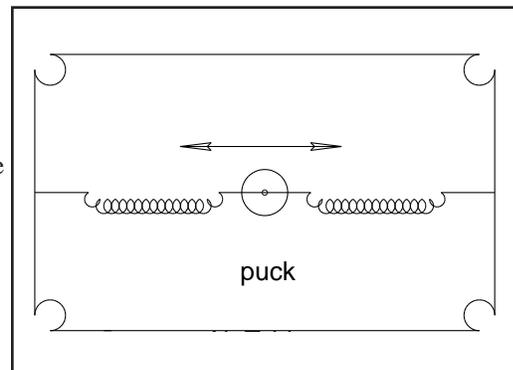
To produce vertical oscillations, only one spring was required. To produce
