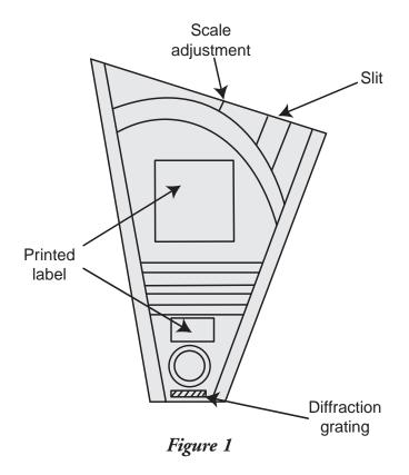
the bulb through the spectrometer. Be careful to aim the slit (on the right side of the spectrometer) at the light bulb and look straight ahead at the spectrum on the scale. You should see a continuous spectrum of colors from red through violet. Mark on the scale below, Figure 1, the colors you see where you see them. Use colored pencils to shade in the observed colors.
